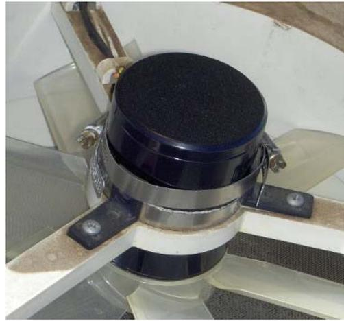
The Shurflo motor has three screws in the shaft end of the motor casing. I could not think of a way to use them for mounting the motor, and since they were not interfering in any way, I just left them in place.
