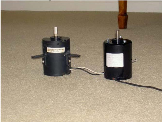
The brackets are required to (1) prevent the motor from falling through the housing, and (2) to prevent the motor from rotating.
